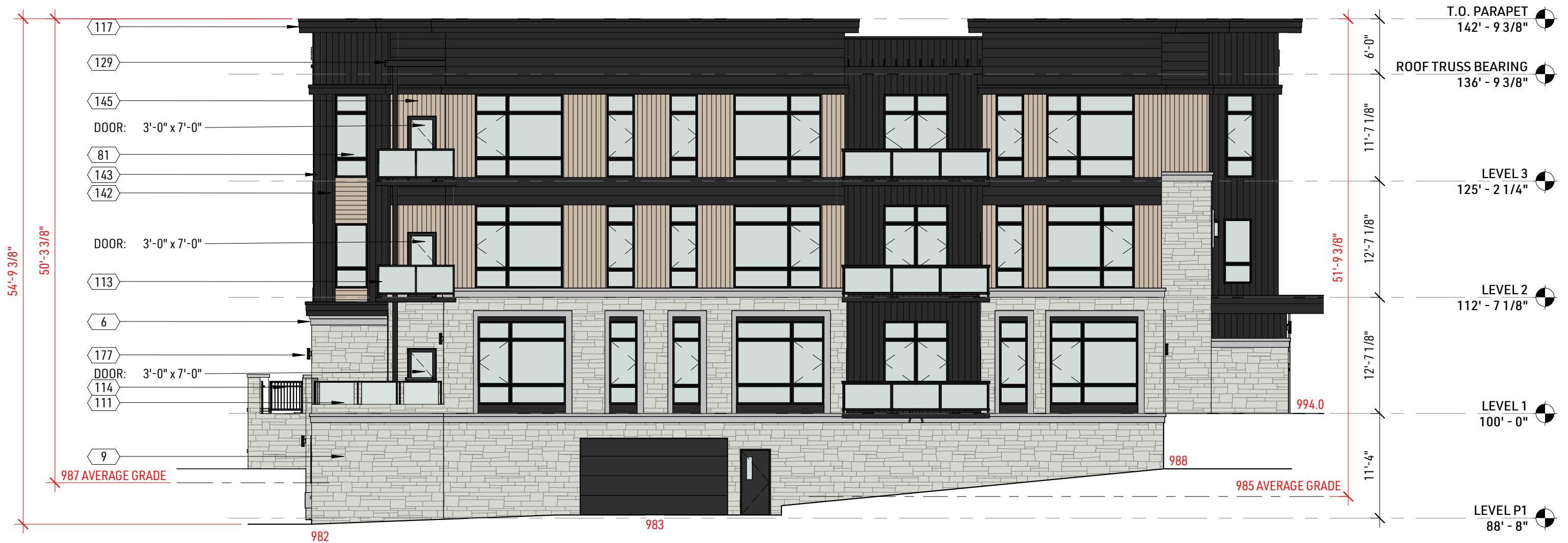
1 EAST EXTERIOR ELEVATION 3/32" = 1'-0"
